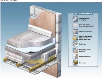
If a separate ceiling is to be installed which will create a void beneath the concrete floor, then the void should be filled with Acoustic Mineral Wool to reduce the possibility of reverberation problems.
