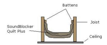
The only trimming required is to reduce the length of the product so that it sits between the joists wall to wall. The edges of the quilt should then be fixed to the joists using battens or upholstery type staples. It is important the quilt is perfectly sealed to the joists to reduce air and sound leakage.
