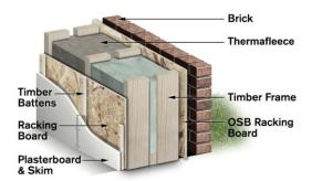
The twin frame system ensures that no thermal bridging occurs within the construction helping maximise insulation performance. By using two 89mm structural timber frames, the width of the construction can be varied to achieve specific insulation performance.
