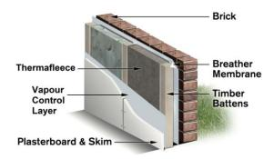
Fit the insulation layers between studs ensuring all joints are close-butted to avoid air gaps. Overlap additional layers to reduce thermal bridging and air gaps. The friction of the insulation should hold it in place.
