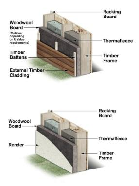
Unlike traditional timber frame systems, the racking board is positioned to the inside of the timber frame. The external insulation attached to the timber frame maintains the frame above the dewpoint temperature reducing the risk of condensation. Additional benefits include low environmental impact, lightweight structure and improved insulation and airtightness.
