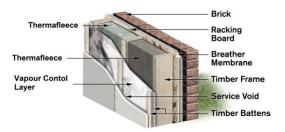
Fix VCL to the warm side of the insulation to reduce the risk of interstitial condensation. The addition of vapour impermeable materials must be correctly detailed and materials must be completely sealed to ensure that no moisture can penetrate into the structure.
