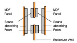
If a baffle is constructed then this should also be lined with the insulation supplied as shown on the diagram.
