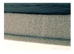
Sound absorbing Mat is used to line the inside of the enclosure. It should be applied with the black film face visible so the adhesive is applied to the grey foam side only.
