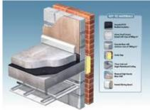
The insulation can be trimmed down to floor level once the screed has cured. With both timber suspended and concrete floors, dot and dab wallboards should only be installed after the floating floor has been laid and as with the skirting boards, the wallboards should not come into contact with the floor.
