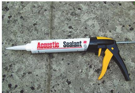
Seal all gaps and holes with Acoustic Sealant and tool smooth ready for decorating when cured
